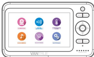
2) Select the channel to be paired, press **OK** to confirm, select
